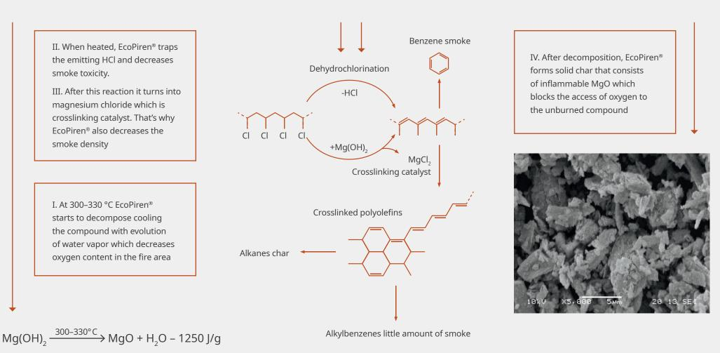
EcoPiren<sup>®</sup> introduces a 4-stage mechanism of flame retardancy to PVC
